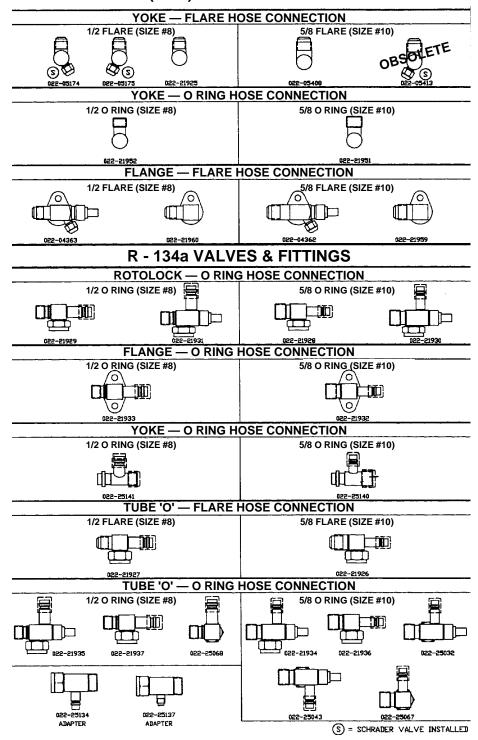
NOTE: SIZE #8 O RING HOSE CONNECTION = 3/4" - 16 UNC THREAD SIZE SIZE #10 O RING HOSE CONNECTION = 7/8" - 14 UNC THREAD SIZE
