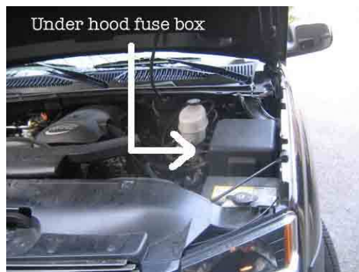
Pic 4 – Fuse Box Location
