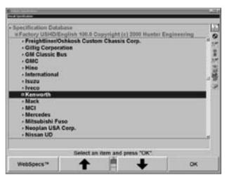
A customized HD specification data base supports most vehicle manufacturers by simply scrolling to the specific model being aligned.
