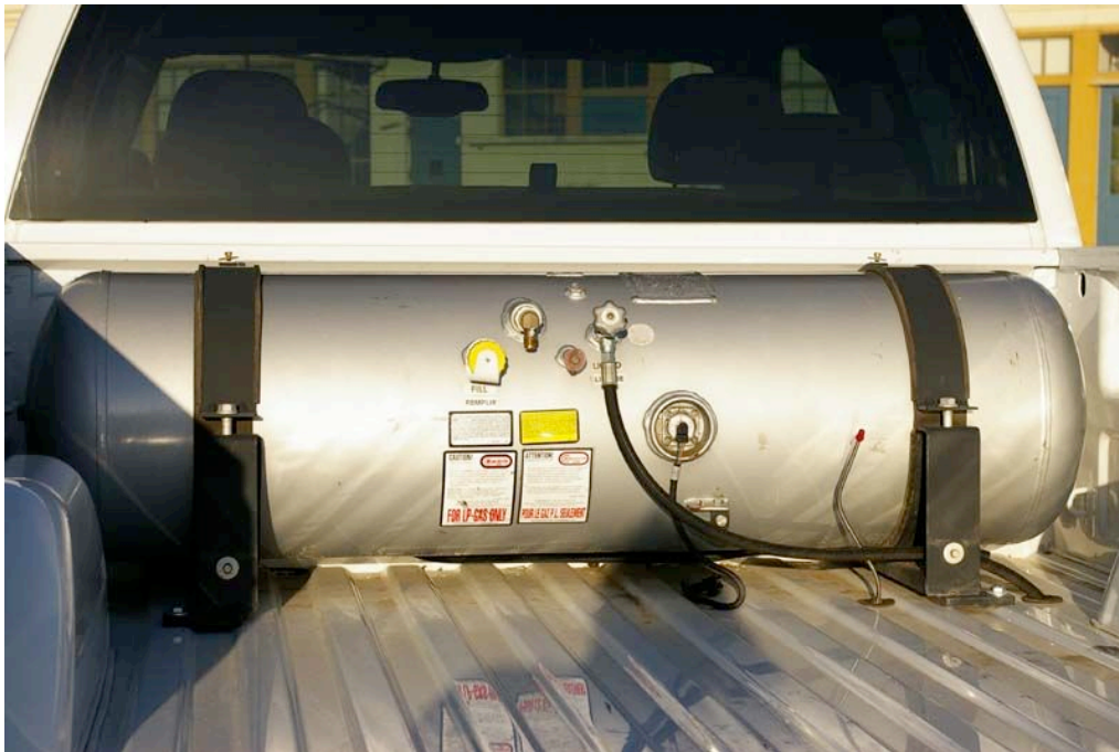
Figure 7 60 Gallon Propane Tank Mounted in 6.0L Vehicle Pick-Up Bed
